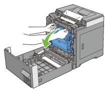
4 Lift the levers at both ends of the fuser, and remove the jammed paper. If you are still unable to remove the paper, go to the next step.
